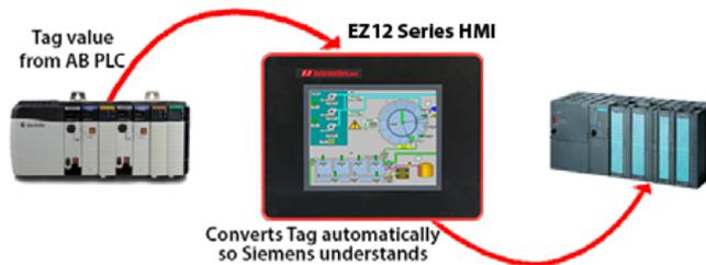
If using Ethernet dual protocol then you can communicate with multiple PLCs of the same type that enables pass-through communication between these different PLCs using the EZTouch HMI®. For example, you can have a MicroLogix, CompactLogix and ControlLogix all transferring data between each other through the EZTouch®. This pass through communication and expressions allow for multi-PLC conditional coding as well.
